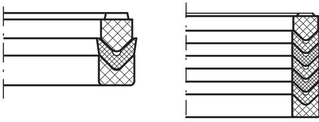
Multi-part roof packing sets are also lip seals. With these seal sets other friction and force conditions set in, caused by the multi-lip, relative long seal design.
