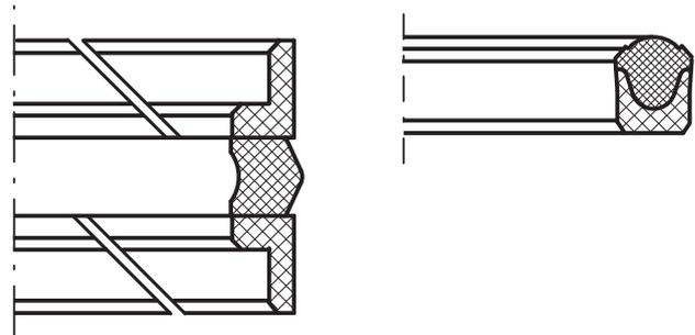
Compact seals can be designed as rod and piston seals.
