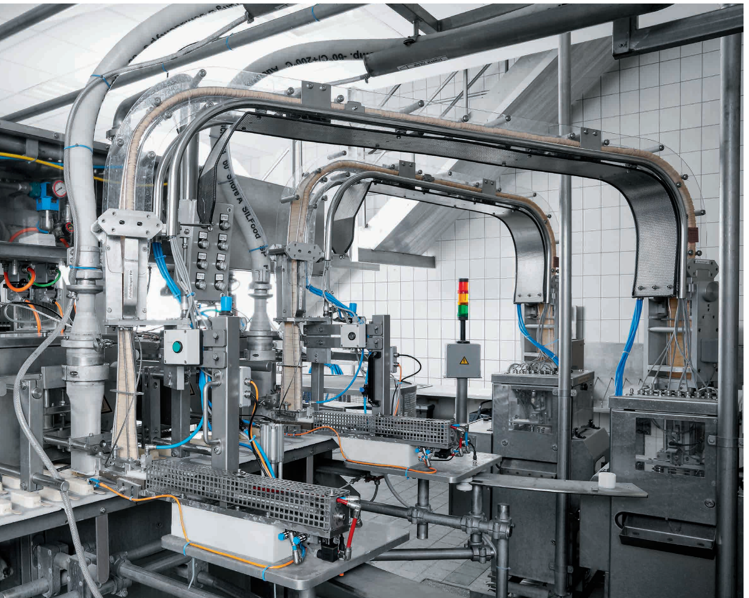
Delicious ice-cream produced sustainably. The MSE6-E2M shuts off compressed air supply if the system comes to a standstill and helps to further reduce consumption by means of efficient condition monitoring.
