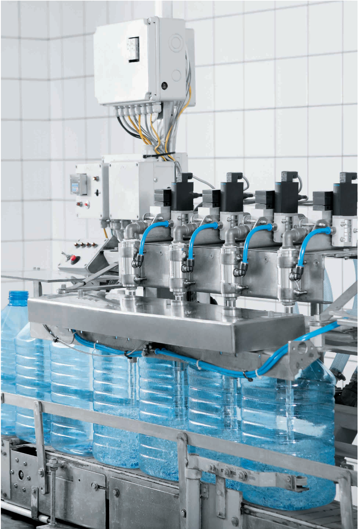
Quick and precise filling of the 5-litre bottles with the solution from Festo. Highlights: the pinch valve VZQA and the fast-switching valve MHE4.
