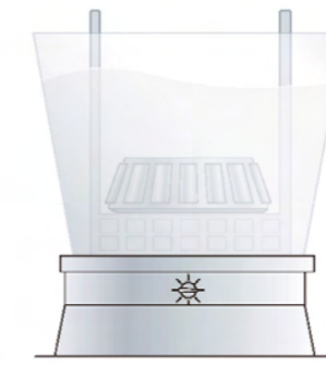
Bearings can be heated in a pan or metal container filled with oil
